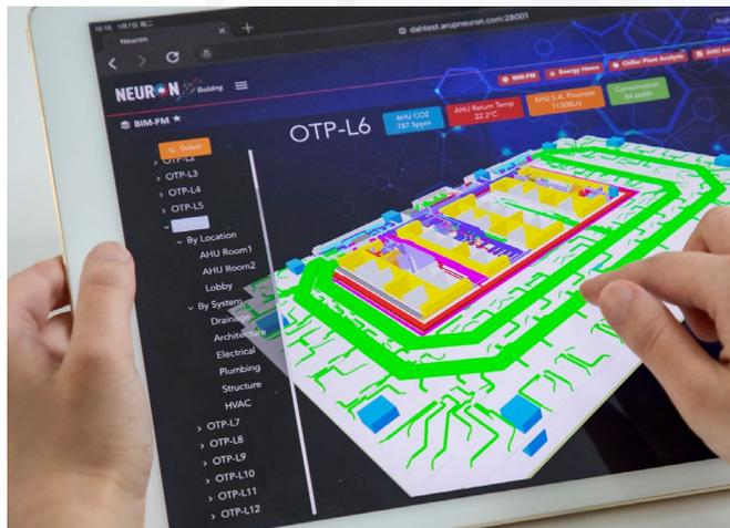
Arup invented the Neuron smart building platform by integrating ‘BIM + IoT + Analytics’ to provide insights to enhance building energy efficiency.
