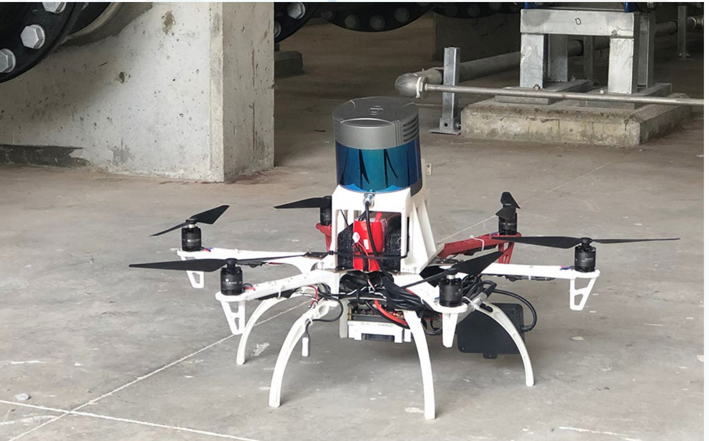
Unmanned Aerial BIM Converter (UABC) generates BIM models based on a drone and indoor 3D laser scanning
